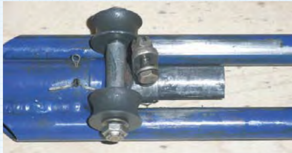
Right or wrong? (1) This picture shows the modified control system well... the only problem is that the roller assembly has been fitted the wrong way round. As fitted, up elevator movement has been severely restricted. (Photo: Tim Wood)
