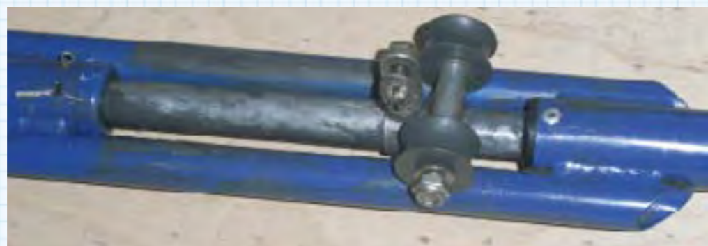
Right or wrong? (2) Here the rollers are the right side of the lower link attachment. This sort of information is often lost to history; it certainly took me a long time to work out what was actually going on. Very well done to Tim Wood (and, of course, Tony Hewitt) for getting to the bottom of this problem. (Photo: Tim Wood)
