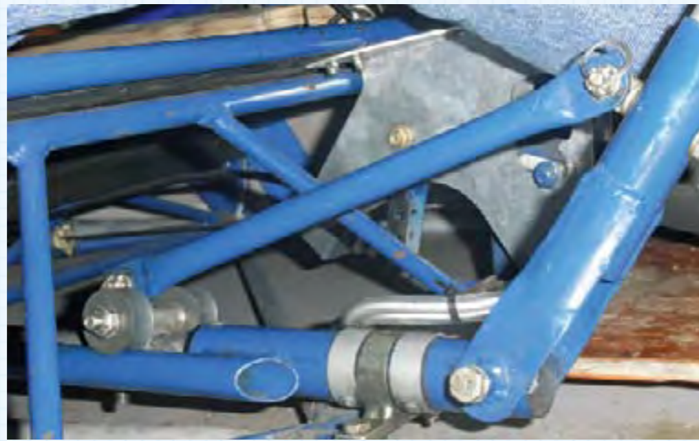
Here is a picture of the general installation of the control stick on Tim's Rans S-10; the rollers have been refitted correctly and no longer restrict the up elevator movement. (Photo: Tim Wood)
