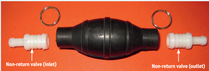
Left and above: here is the Kimpex fuel primer bulb that caused a restriction in the fuel supply on the Rans S10. The primer consists of a squeezable rubber bulb and two non-return valves (NRV) to control the direction of flow. (Photo: Malcolm McBride)
