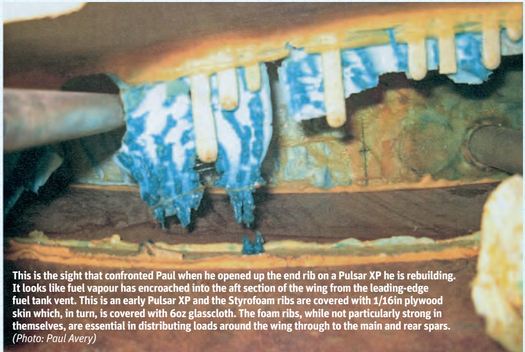
In addition to providing a solid structural base for the wing skin, the Styrofoam ribs also support the primary control push/pull rods. This picture of a Pulsar XP failed rib shows a (now unsupported) flap drive bearing. (Photo: Paul Avery)
