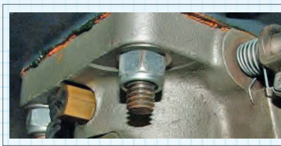
Here's a close-up of a carburettor flange from a picture I featured in December's Light Aviation . LAA Inspector Robin Dispain wrote to me pointing out that gasket sealant had been used during the assembly and that this shouldn't have been necessary. Robin made a good point, which I promised to share. If there's excess sealant on the outside then there's a good chance that there will be excess on the inside. Food for thought! (Photo: Barry Smith)
