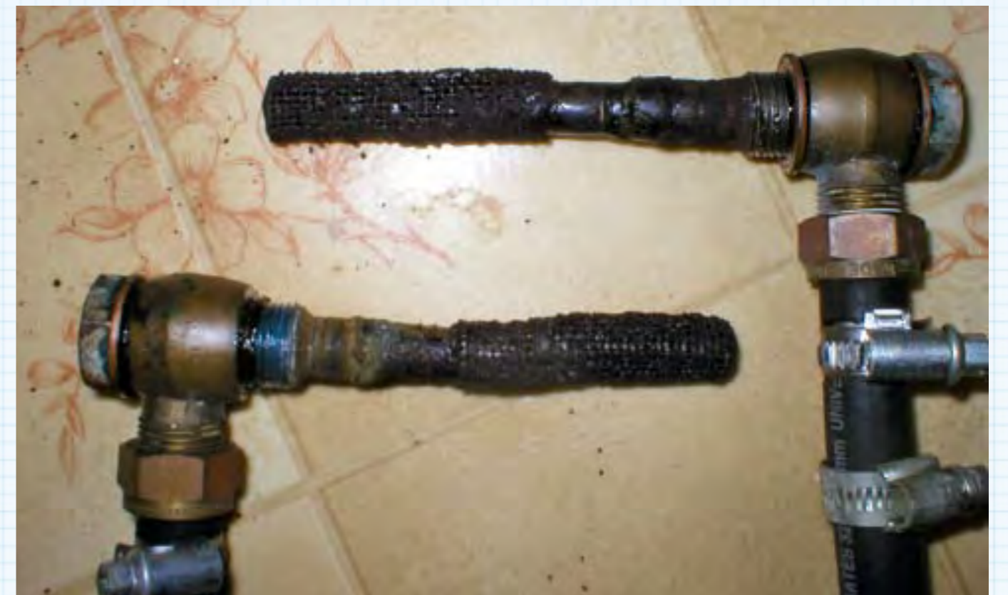
Who would have thought that, after only ten years of standing in a hangar, fuel would have more or less written off the fuel tank outlet filters in Keith's Pietenpol? (Photo: Keith Hodge)
