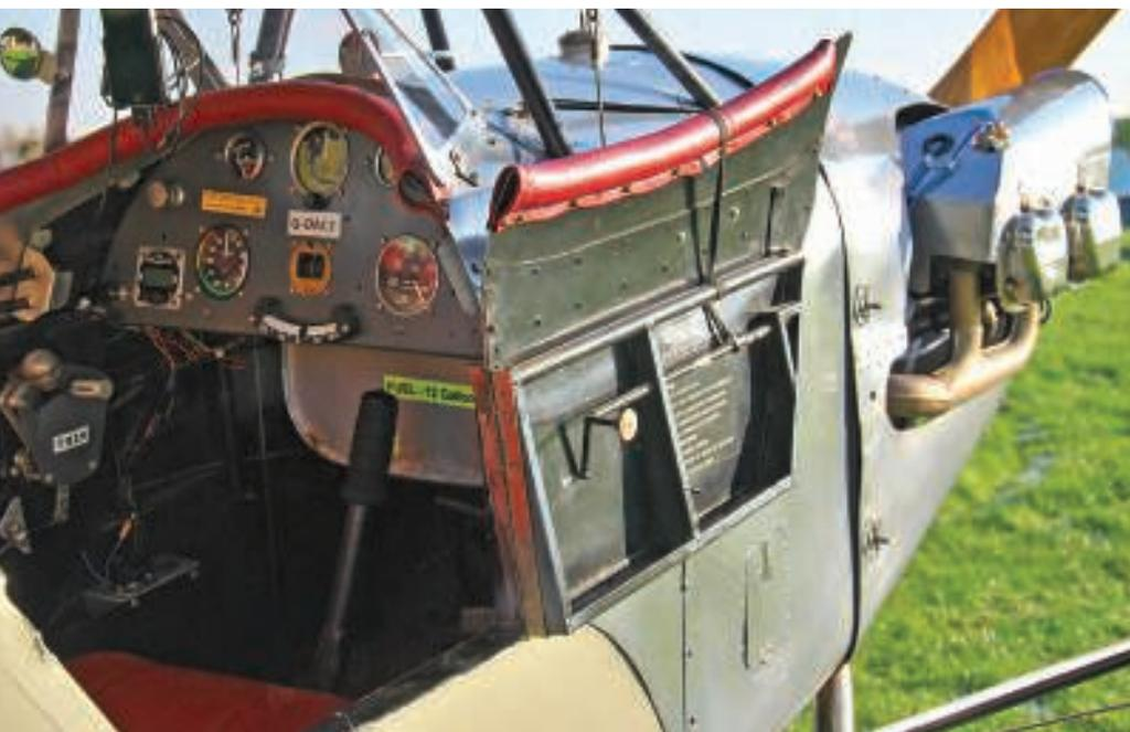
(Above) As you'd expect, for many modern pilots, the Baby Ace's cockpit is something of a snug fit, but facilitated by a small, forward-hinging door, which latches against the fuselage. Unwisely, Clive ignored Gerry's advice, which made his entry much trickier!
