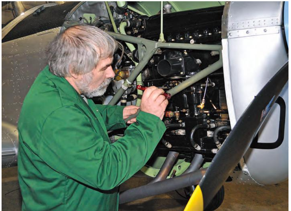
Alan Turney inspects the throttle linkage on a Chipmunk. Is the wire locking secure, and has it been done correctly?
