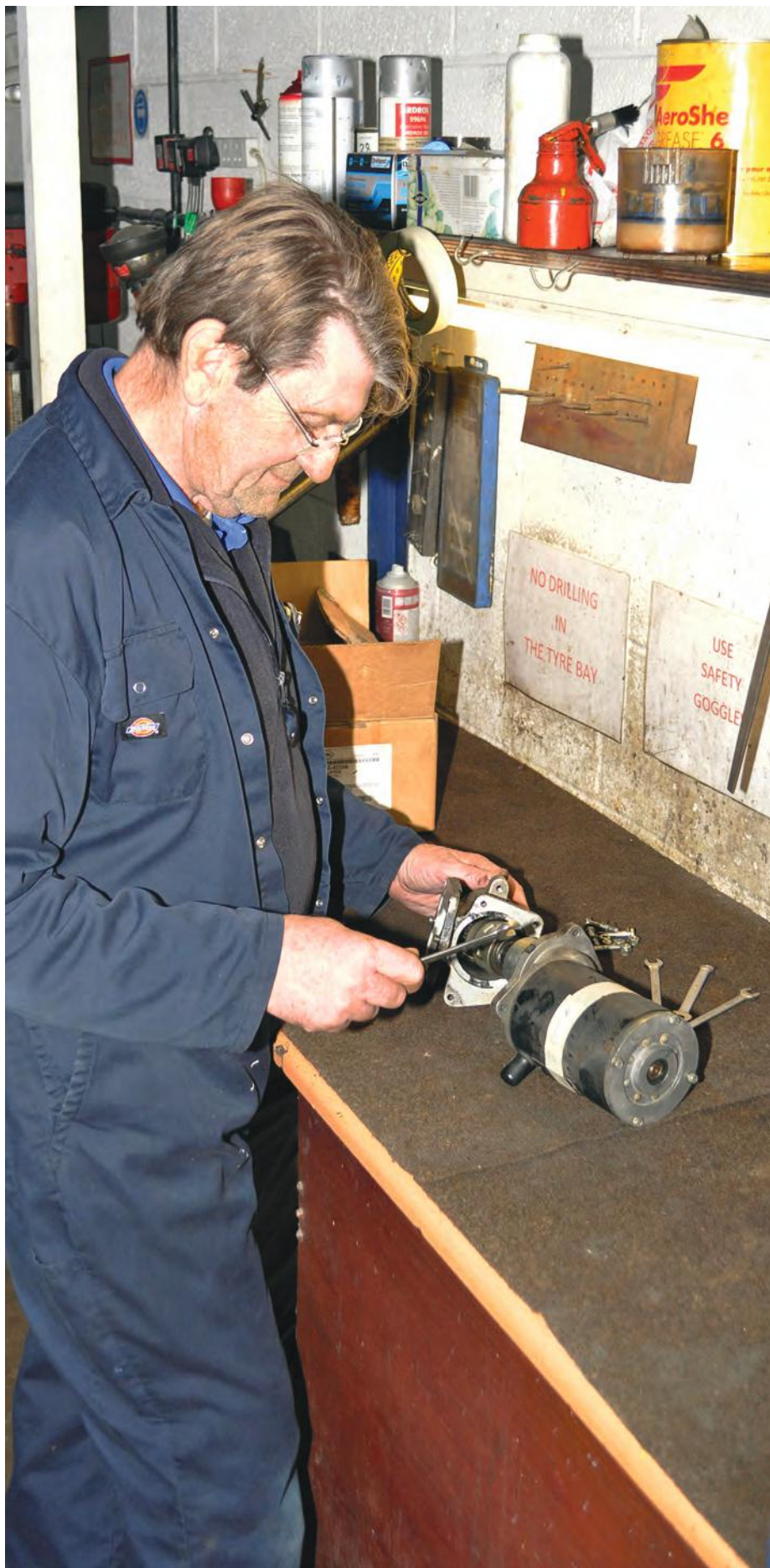
I suspect most people don't check their generator until it stops charging! A deep inspection of the electrical system at say, three yearly intervals, could include cleaning and inspecting the generator.
