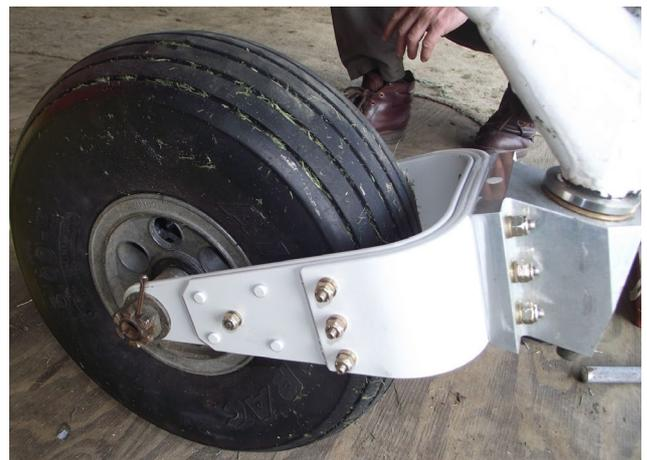
Fig 2. The picture above shows a strengthened (three-leaf) fork. This component is now available to CZAW SportCruiser owners and can be fitted under an LAA Standard Modification (SM 13680).
