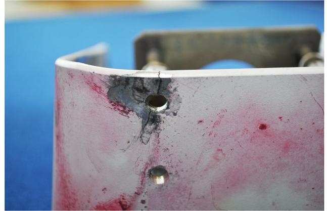
Fig 1. This close-up of the mating face of a two-leafed (original type) fork showing cracks radiating from an attachment bolt hole. These cracks cannot be seen until they reach the outside edge of the fork without the fork being dismantled from the assembly. This is particularly worrying with regard to the lower crack should it propagate unseen between the attaching bolt holes as it could lead to a sudden and unexpected failure of the fork.
