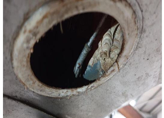
Fig. 1 Who knows what you might find lurking inside your aircraft after a relatively long lay-up – the owner of this aircraft wouldn't have spotted the wasp nest if he hadn't taken the time to remove the panel and take a look.
