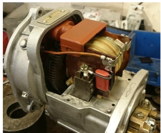
Fig 2. This picture shows the rewound (modified) coil as fitted to the M-14P magneto: note the modern metallised polyester film capacitor bonded to the side of the coil-winding end plate, this replaces the troublesome varnished paper type originally used. This minor modification, which effectively employs automotive technology, is now approved by the UK CAA and, in turn, EASA.
