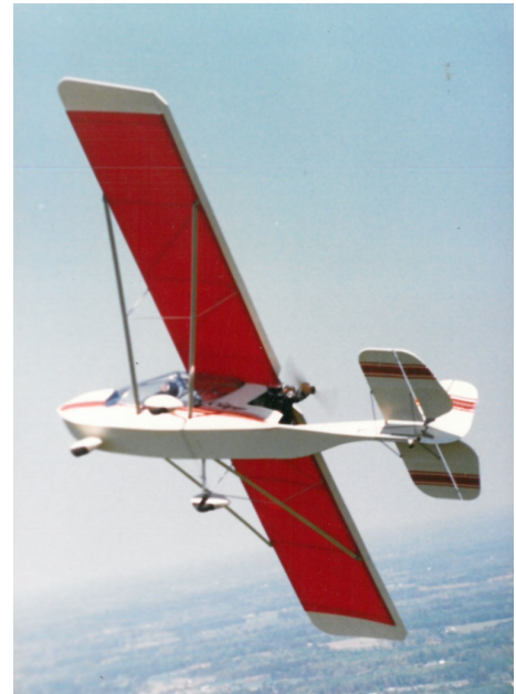
Fig.1 The Challenger is a high wing, tricycle gear, pusher engine, kit-built microlight aircraft. In the UK some 50 aircraft are listed as LAA Permit to Fly aircraft with a small number having transferred to the de-regulated microlight category (SSDR).
