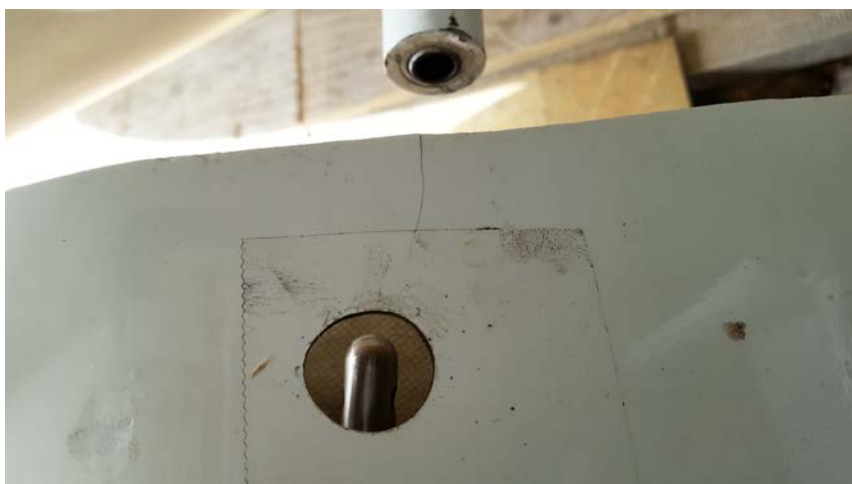
Fig. 1 This picture shows the flap drive pin visible through the viewing hole in the upper surface of the flap, the hole is there for lining-up purposes when rigging the aircraft.
