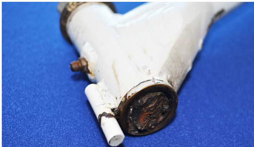
Fig. 2. The broken CZAW Spindle
