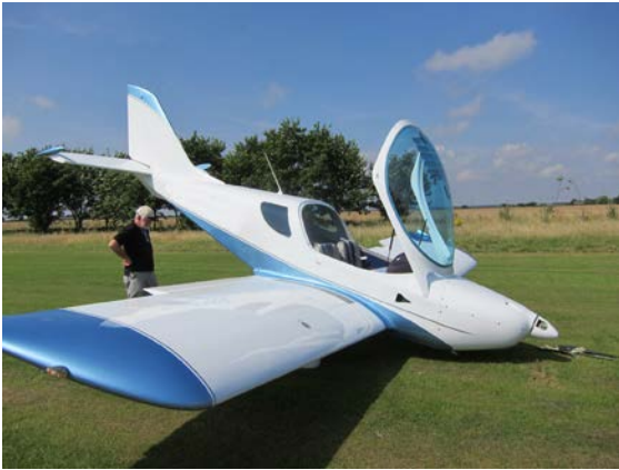
Fig. 1. This CZAW SportCruiser suffered a nose undercarriage Spindle assembly failure at low speed.
