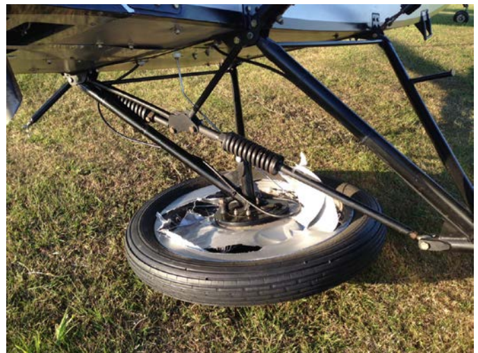
Fig. 1. In this example the starboard lower rod end has failed. The port rod end, which can be seen connecting the spring strut to the axle assembly, remains intact.
