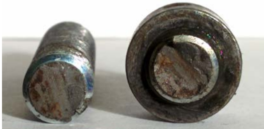
Fig. 2. Clear signs of fatigue in the failed bolts suggestive of looseness in service.
