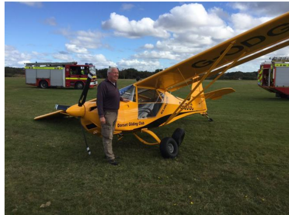
Fig. 1. The pilot of this Eurofox did a good job of getting the aircraft down without further damage after the undercarriage attachment bolt failed.
