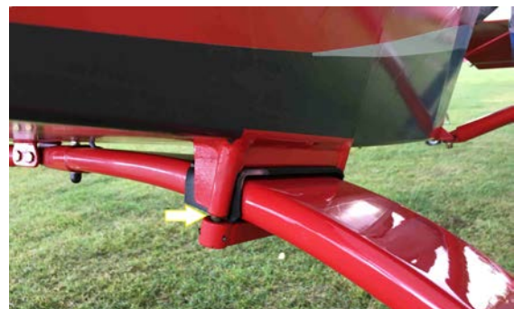
Fig. 3. The arrow marks the positions of spacing washers required so that the attachment bolt can be tightened more firmly.
