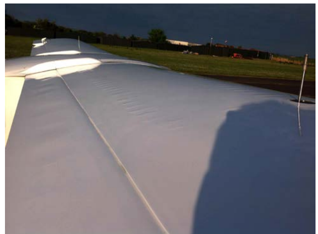
Fig 2. Though difficult to see in this picture rippling can be seen in the top surface of this J400 wing. The recent AIL withdraws any previous approval for Mogas use.
