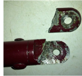
Fig. 2 This picture from the LAA library shows a failed 'original design' strut end fitting.
