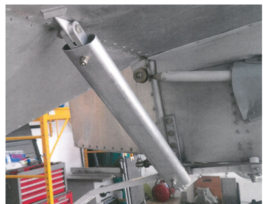
Fig. 4 The latest strut design – note that the end fitting is bolted rather than riveted in place.
