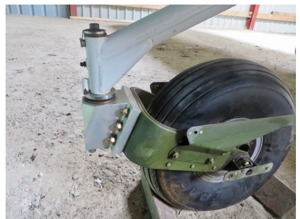
Fig. 2 The picture above shows the prototype spindle assembly attached to a strengthened CZAW undercarriage leg. Note that the spindle assembly is subject to an annual inspection requirement (see LAA/MOD/338/019 Issue 1) and the fork, here a two-leafed variant, is subject to inspections laid out in LAA/MOD/338/016 Issue 2.
