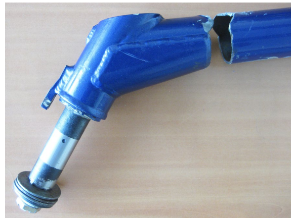
Fig. 1 This picture shows a failed PS. Mk. 1 undercarriage leg.
