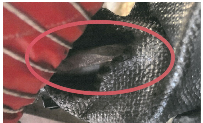
Fig 2. This steering control rod is, in service, hidden by a protective 'boot' in place to protect occupants from dangerous fumes in the engine compartment. It is essential that 'hidden' parts like this are subjected to a close inspection as part of the aircraft Tailored Maintenance Schedule (TMS).
