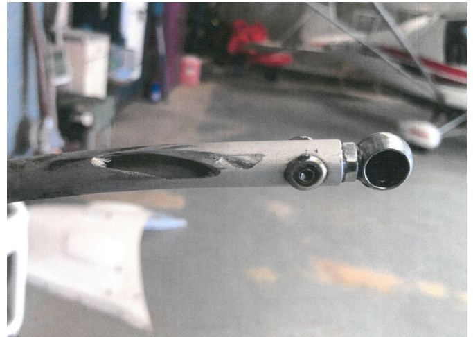
Fig 1. If a steering pushrod like this one actually failed during a take-off or landing it could lead to a loss of control accident or incident. Though not (in this case) part of the aircraft primary flying control system it does perform a critical role in the ground control system pathway and therefore deserves a regular and detailed inspection.
