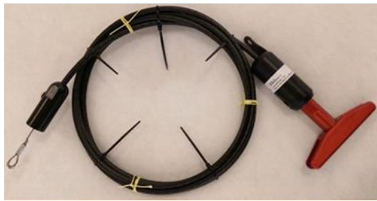
Figure 3 Activation handle (image courtesy of BRS Aerospace) and Warning placard
