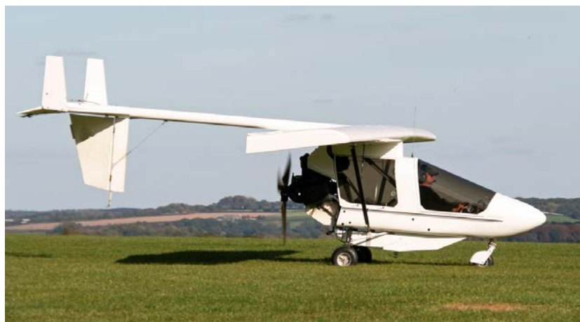
Fig 1. An example of an LAA Administered Streak Shadow aircraft; this picture shows clearly the main fuel tank attached below the engine and the 'slipper' tank attached between the mainwheels to the fuselage floor.
