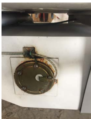
Fig 2. Access for internal inspection of the 'slipper' tank is gained by removing the fuel sender unit, though care is needed to ensure that the unit is completely resealed during refitting
